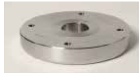
GP40205 Airline Ball Valve Weld-In Tank Pad 4 x M10 Blind-tapped holes on 103.4 PCD
